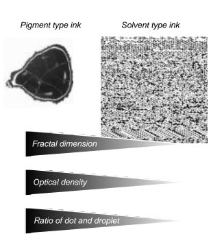
Figure 7. The difference of printed dot form on PPC paper
